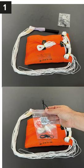
**EN** Prepare the rescue over a clean, dust-free surface, and make sure the lines are not tangled.
