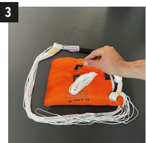
Remove the lark's head knot of the rubber band and also remove the rubber band from the webbing loop.
