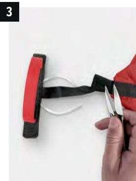
**EN** Cut and remove the stitched line that connects the parachute handle with the container, be careful not to damage the webbing!
