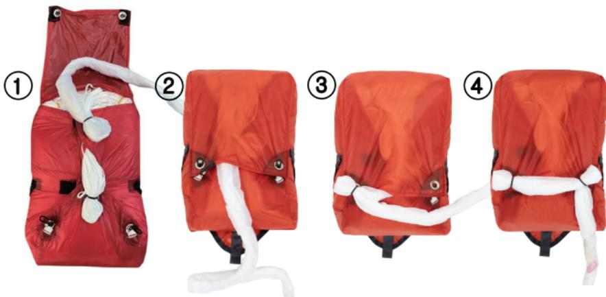
**TEST:** Lifting the bridle, check the force required to allow the lines to free themselves from the closing loop of the deployment bag. This force should be around 200g. This force may be verified with a spring balance, if available.
