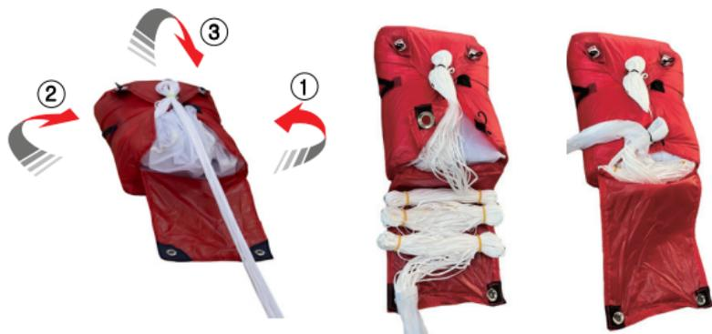
Stow the lower suspension lines in a 'figure of 8' pattern, fixing each pair with rubber bands at each end. Put in lines in the inner bag and close last loop with a bight (3cm loop)
