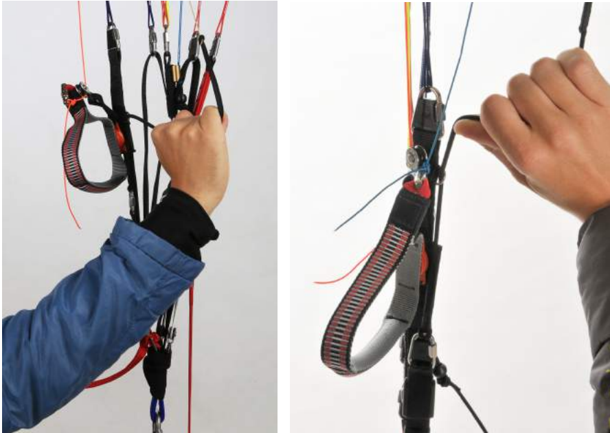
Fig. 5a, b: Steering with wing tip brake
