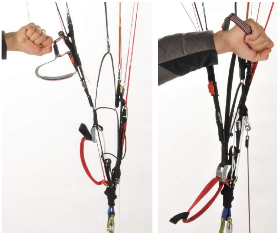
Fig. 4a, b, c, d: Steering with outer 2D steering line only (Trim speed and accelerated)
