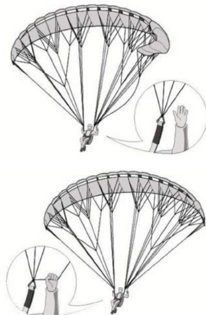
Fig. 7: Grabbing the stabilizer/winglet main line
