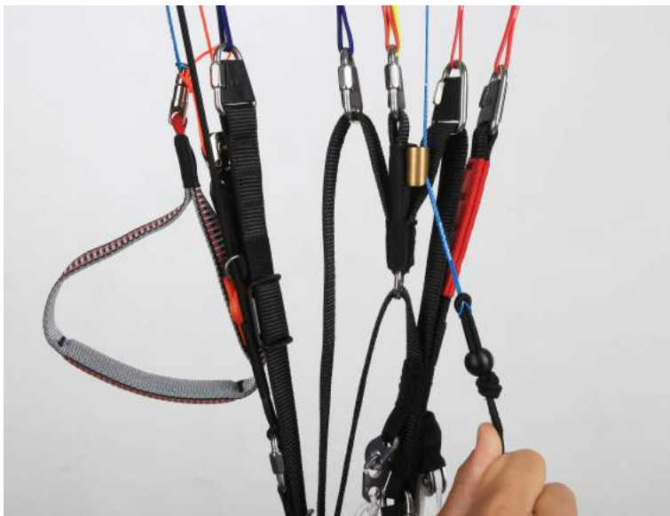
Fig. 14: Activating the Torque compensator
