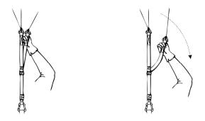
The glider can be steered while in big ears using weight shift alone.
