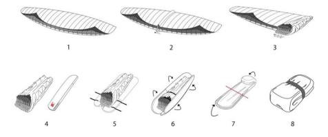
When you fold the glider, don't fold on the part of the profile with Rigifoils but fold on the part of profile where there are no Rigifoils.
