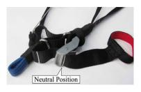
Trimmers should be in the neutral position during launching and landing.
