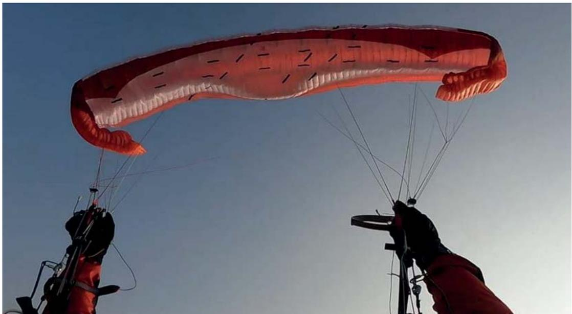
**Figure:** Stable deep stall after a front collapse on the Boomerang 12. The trailing edge of the glider goes up, which stops the glider returning to normal flight.
