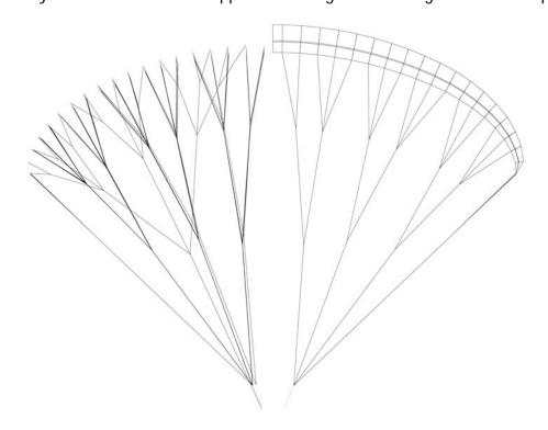
Weight and drag have also been reduced by reduction of the total length of line material used, and the introduction of a new, hi-tech, light fabric.
