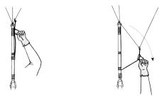
Although the noise of the wind around your ears may indicate the airspeed improves, the airspeed does not improve with big ears. You may use the speedbar in combination with big ears to maintain your forward speed but increase the sink.
