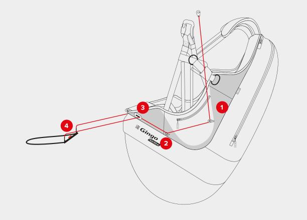
**CAUTION:** Make sure that the speed system is not too short. The front risers of your paraglider must not be pulled down in normal (unaccelerated) flight.
