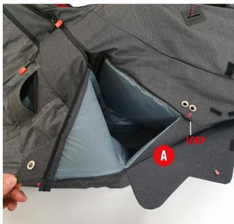
**! WARNING:** When installing the reserve make sure the reserve handle is up and the reserve lines are facing down.
