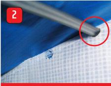
Push the wire through all the front holes on the ribs inside the glider near the top surface.
