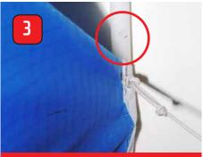
Fix the wire in one side of the plastic bar in the small groove in the bar as shown.
