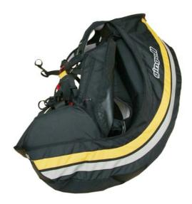
You can add lateral protection to the Gingo II by fitting a pair of GIN side impact plates into the side pockets on the harness, either side of the back protection.
