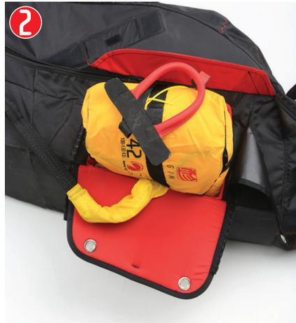
Place the rescue into the bag with the handle attachment facing UP
