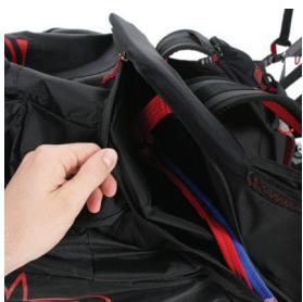
Neatly pack the Y bridle into the bridle tunnel
