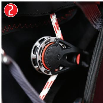
**CAUTION:** Make sure that the speed system is not too short. The front risers of your paraglider must not be pulled down in normal (unaccelerated) flight.
