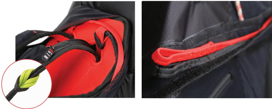
**WARNING:** When connecting the rescue bridle be sure to secure the connection using tape, rubber bands or heat shrink wrap. If the lines are not secure they may burn or cut from excess friction.
