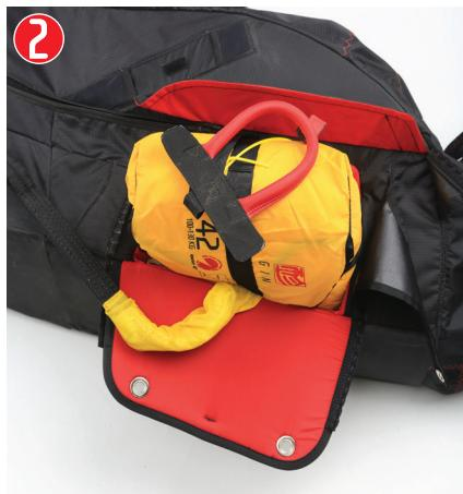
Place the rescue into the bag with the handle attachment facing UP
