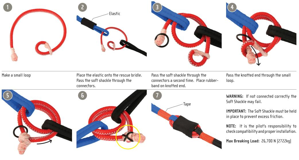
Pull tight to close the loop around the knot.
