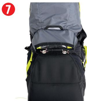
Insert the rescue handle hooks into the eyelets
